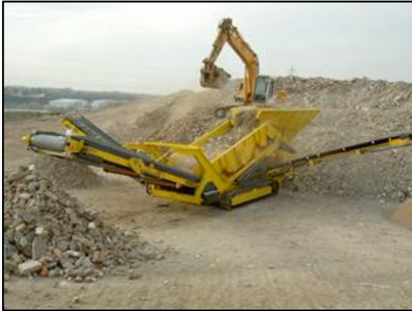
Figure 2.9: Temporary on-site rock crusher
