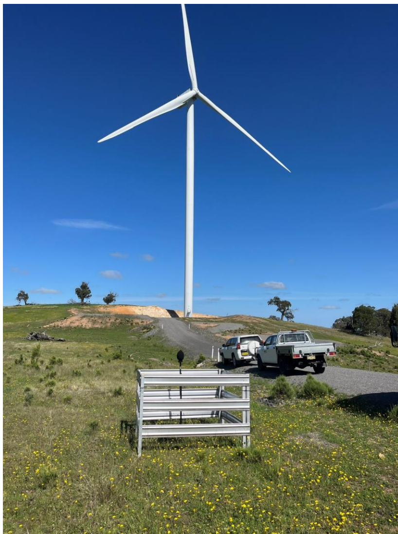
Figure 1: Typical near field monitoring installation
