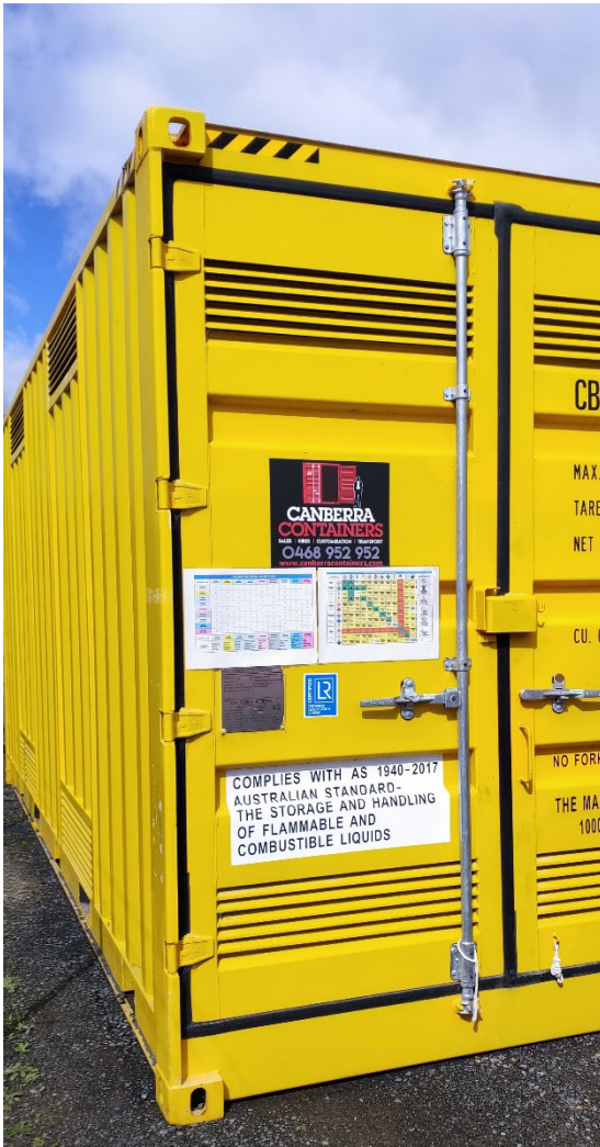
Photograph C.10 Lockable, self-bunded flammable goods storage well managed on site
