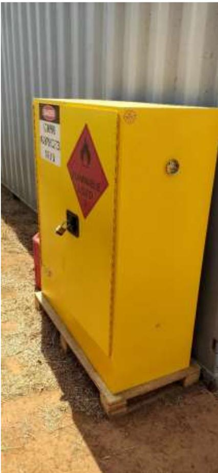
Photograph D.16 Lockable, self banded flammable goods storage
