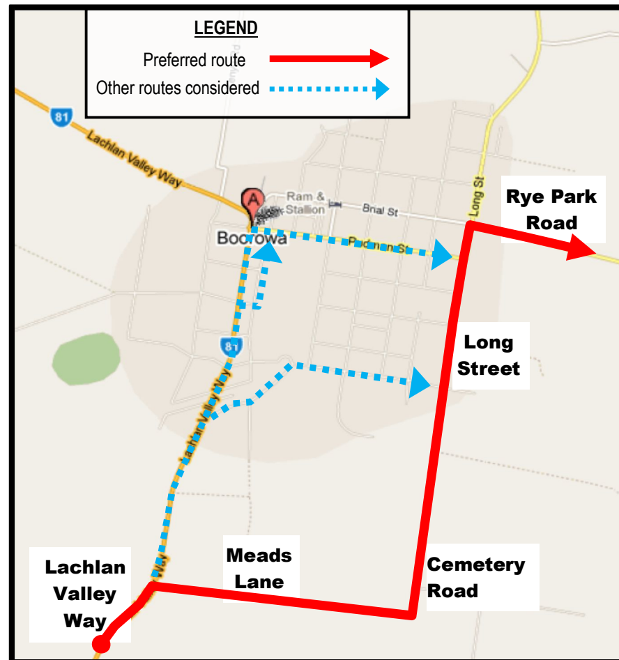
Figure 3.3: Over-Size Vehicle Transportation Route Around Boorowa Town
