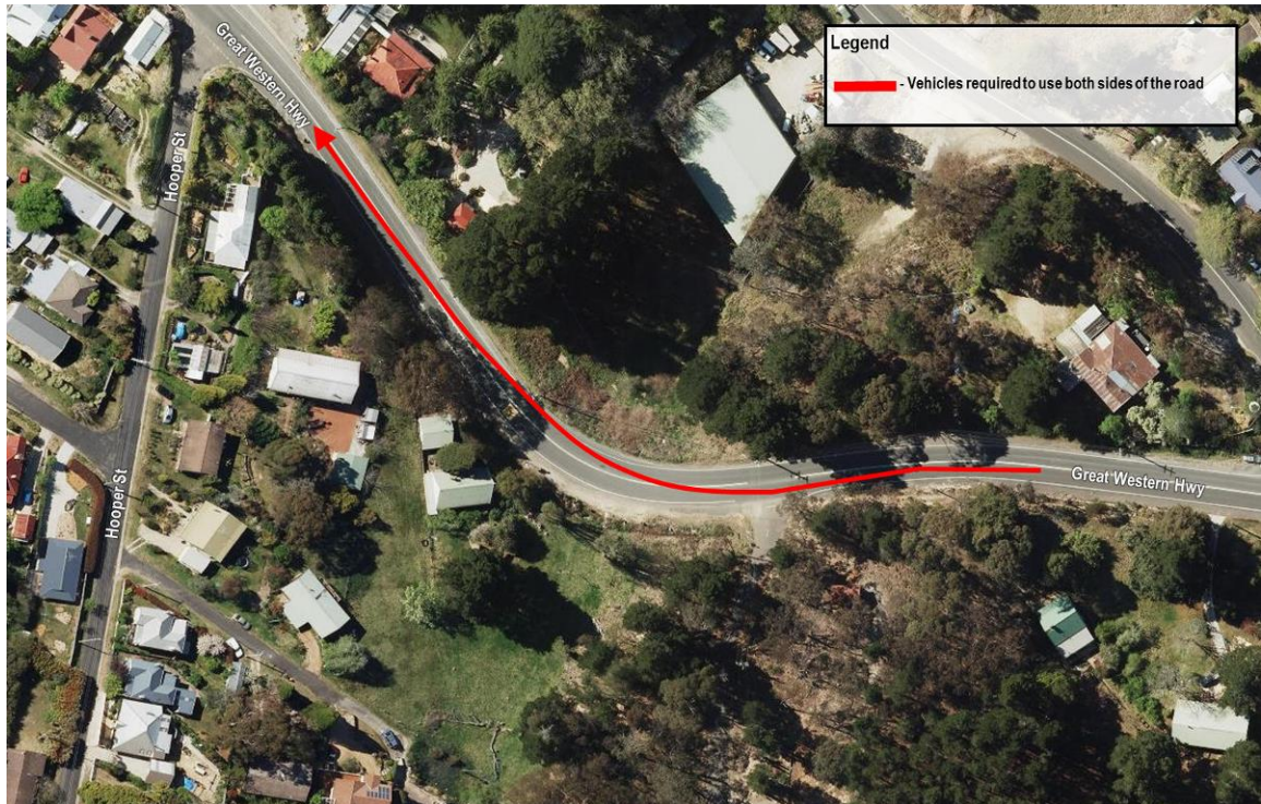
Figure 3.6: Vehicles Use Both Sides of the Road near Mount Piddington Road on Great Western Highway
