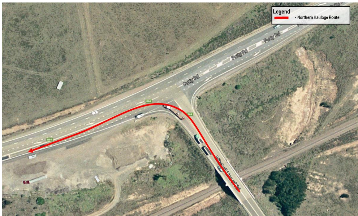
Figure 2.7: Vehicles Use Both Sides of the Road at Golden Highway (Mitchell Line of Rd) / Golden Highway (Putty Road) Intersection
