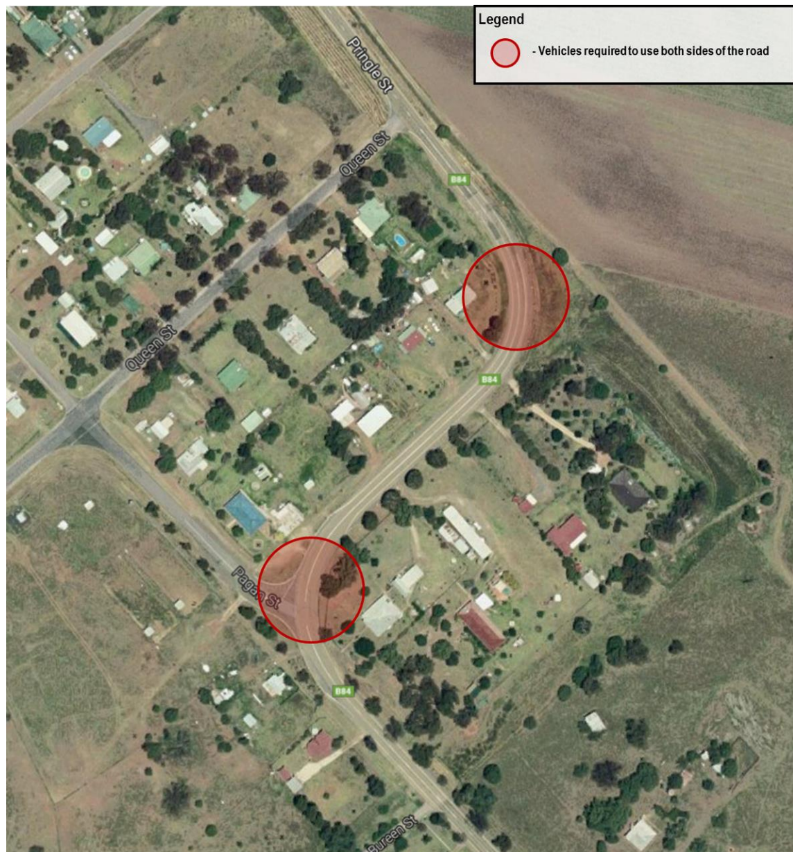
Figure 2.9: Vehicles Use Both Sides of the Road at Jerrys Plains on Golden Highway
