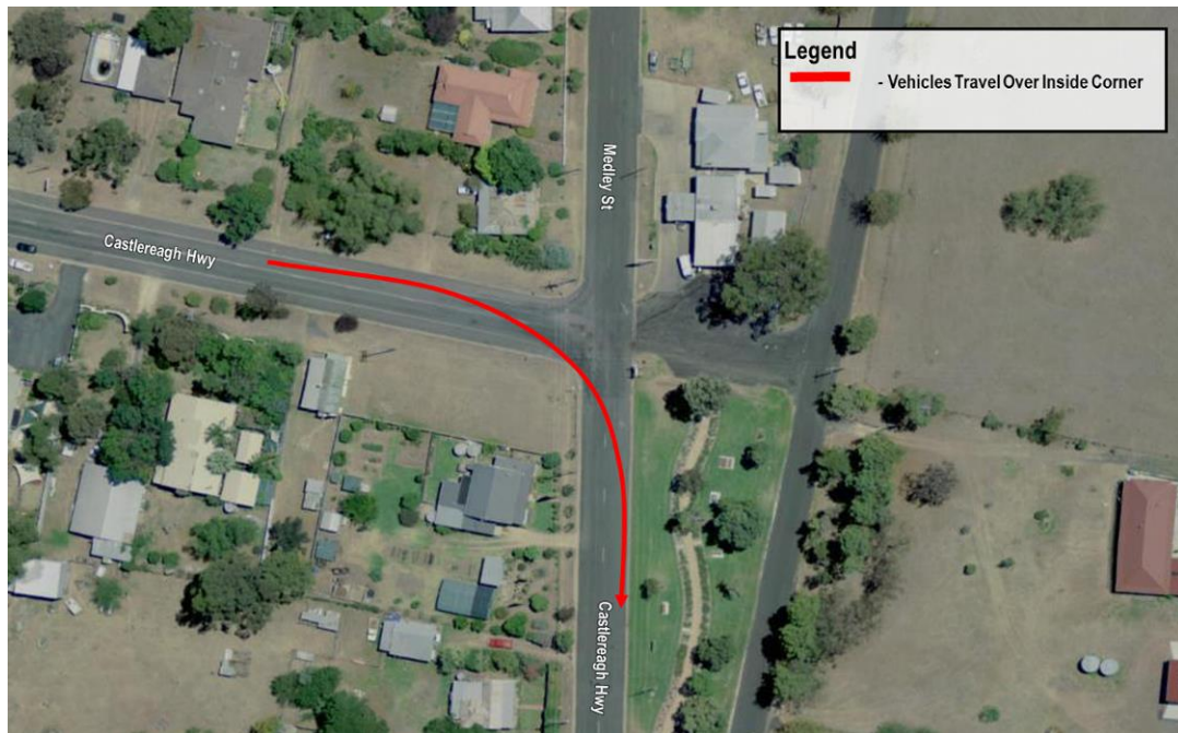
Figure 2.13: Vehicles Travel Over Inside Corner at Castlereagh Highway (Fisher Street / Medley Street) Intersection, Gulgong
