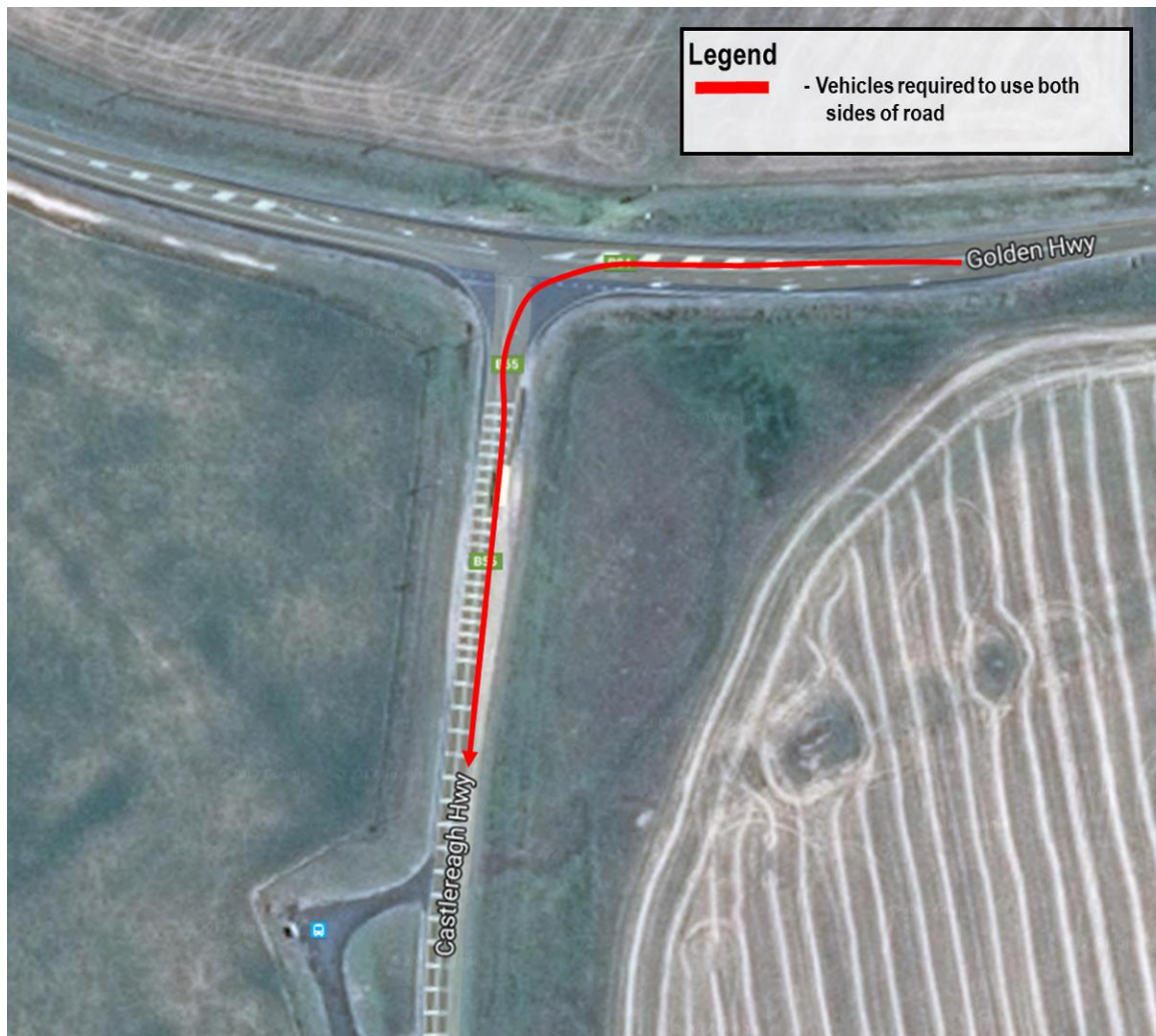
Figure 2.12: Vehicles Use Both Sides of the Road at Golden Highway / Castlereagh Highway Intersection
