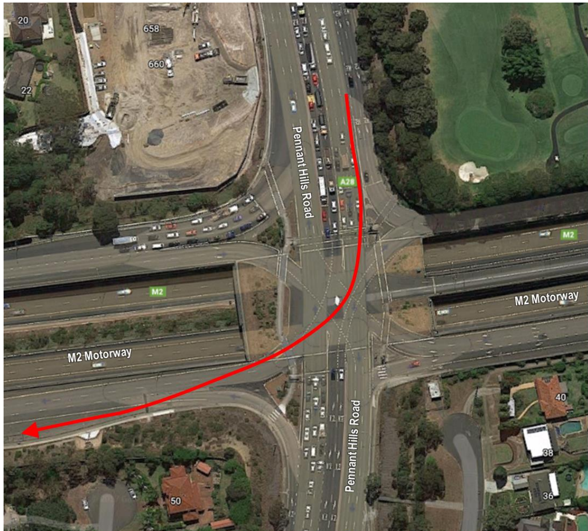
Figure 3.4: Vehicles Use all southbound approach lanes at M2 Motorway / Pennant Hills Road Intersection
