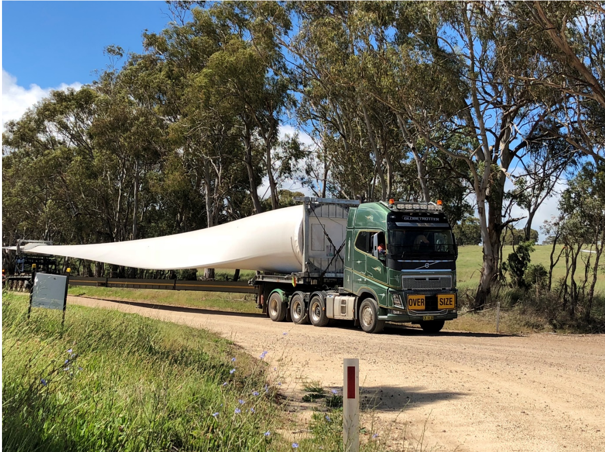
Image 2: Example of an Extendable Trailer in use at Sapphire Wind Farm
