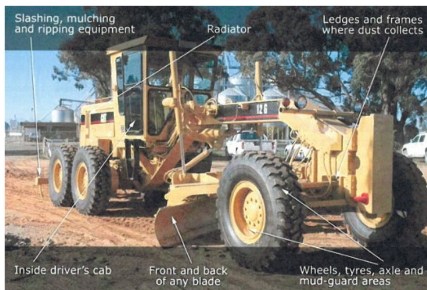
FIGURE 5-1 EXAMPLE OF CRITICAL CONTAMINATION AREAS REQUIRING THROUGH CLEANING (CIVIL CONTRACTORS FEDERATION, 2010)
