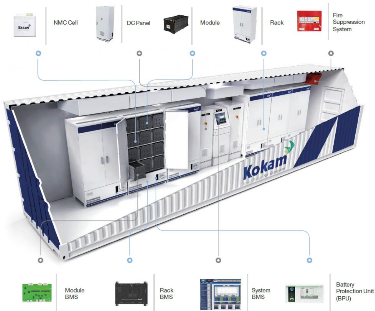
Figure 3: An indicative containerised battery energy storage system © Kokam
