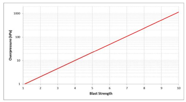
Figure 6-1: Theoretical Peak Overpressure [7]
