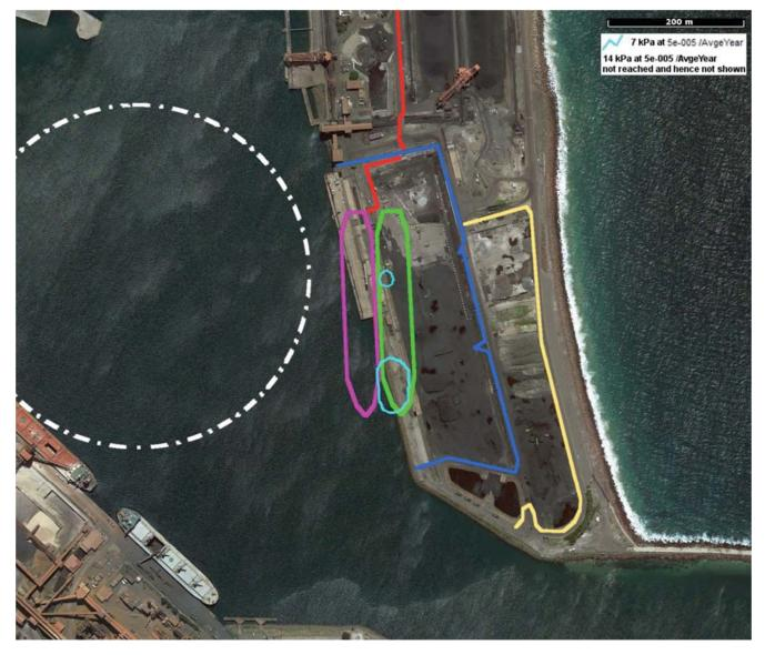
Figure 9-4: Propagation and Injury Risk due to Explosion Overpressure
