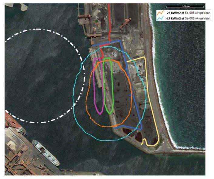
Figure 1-2: Propagation and Injury Risk due to Heat Radiation
