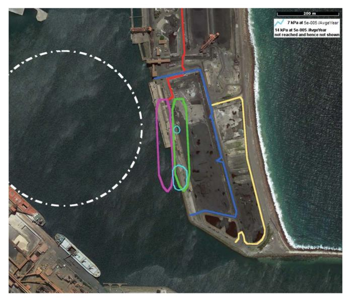
Figure 1-3: Propagation and Injury Risk due to Explosion Overpressure
