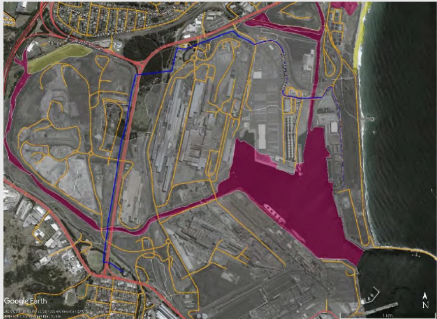
Figure C - Wollongong 1:25,000 Acid Sulfate Soil Risk Map extract showing pipeline alignment (blue line)
