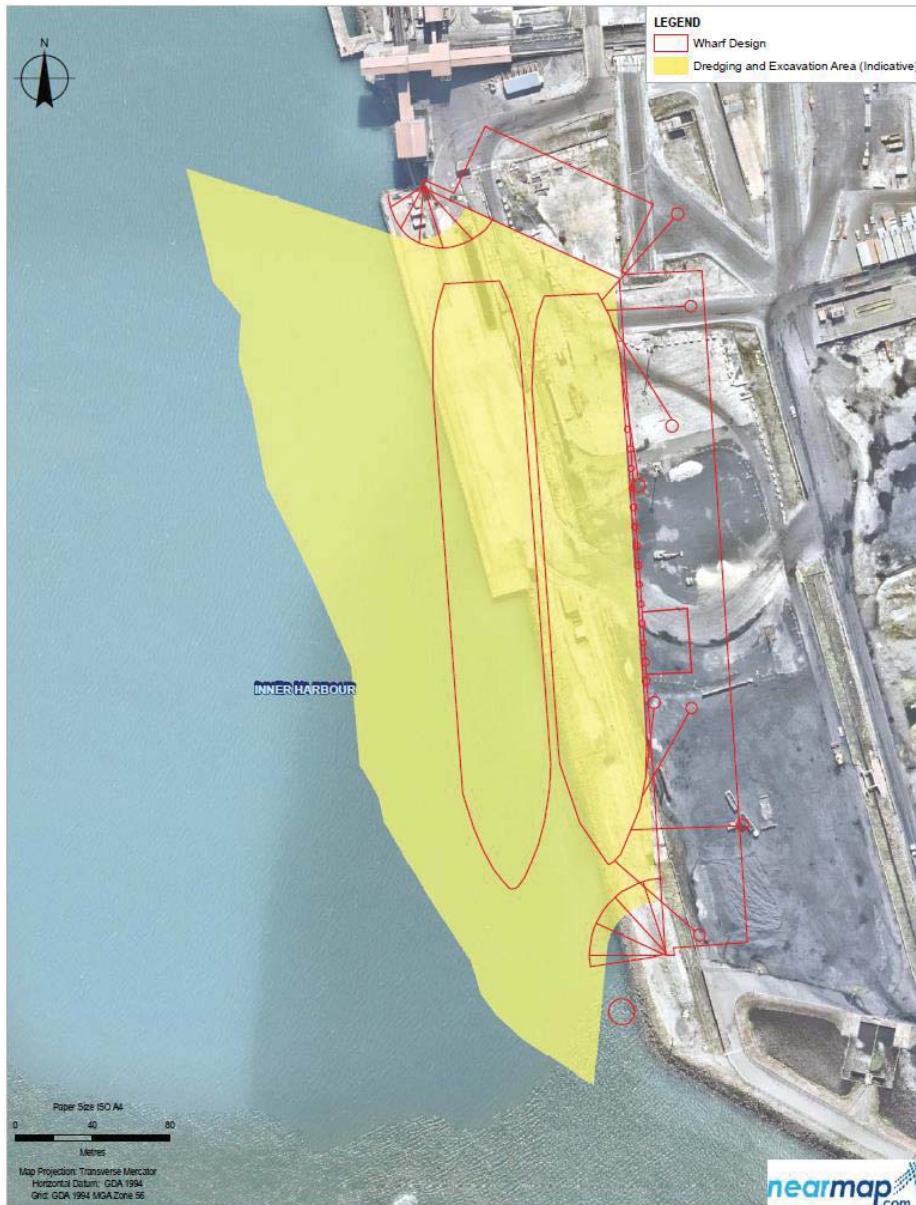
Figure 1 Excavation and dredging area
