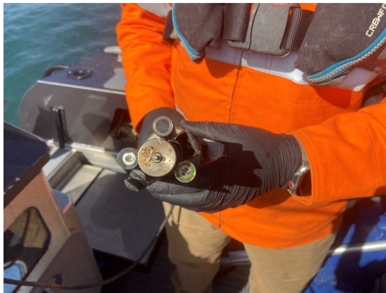
Sensors of EPL 1 removed from the water for cleaning. Photograph taken 11:20 am on the 18 th August 2023.
