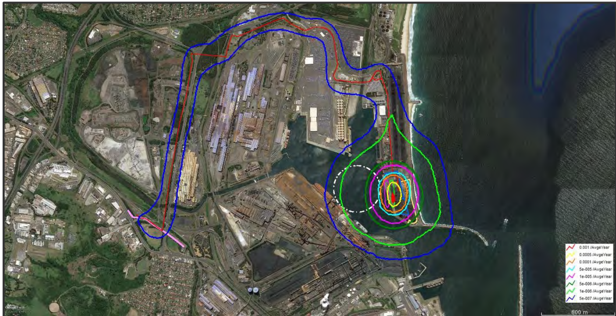
Figure 7 | Fatality Risk Contours- Pipeline and Berth
