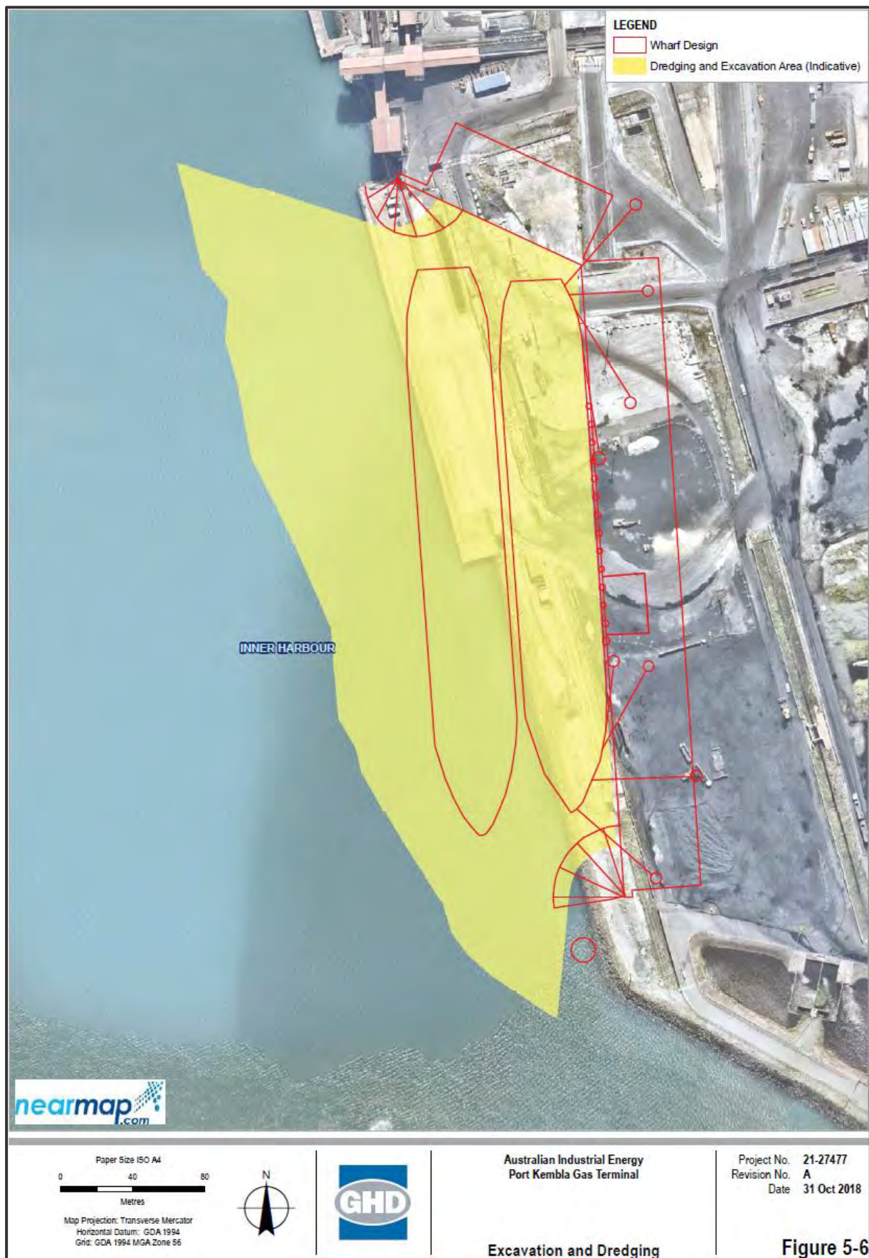
Figure 4 | Area to be Excavated and Dredged
