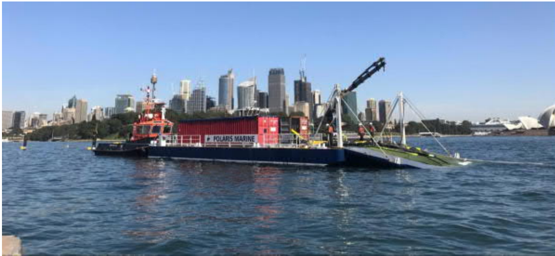
Figure 6-12 Silt Curtain Installation Barge
