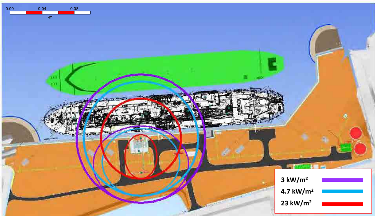
Figure 8-1: Scenario 6, 25mm Jet Fire Thermal Radiation Impacts at ORF (1m above grade) – Initial Conditions
