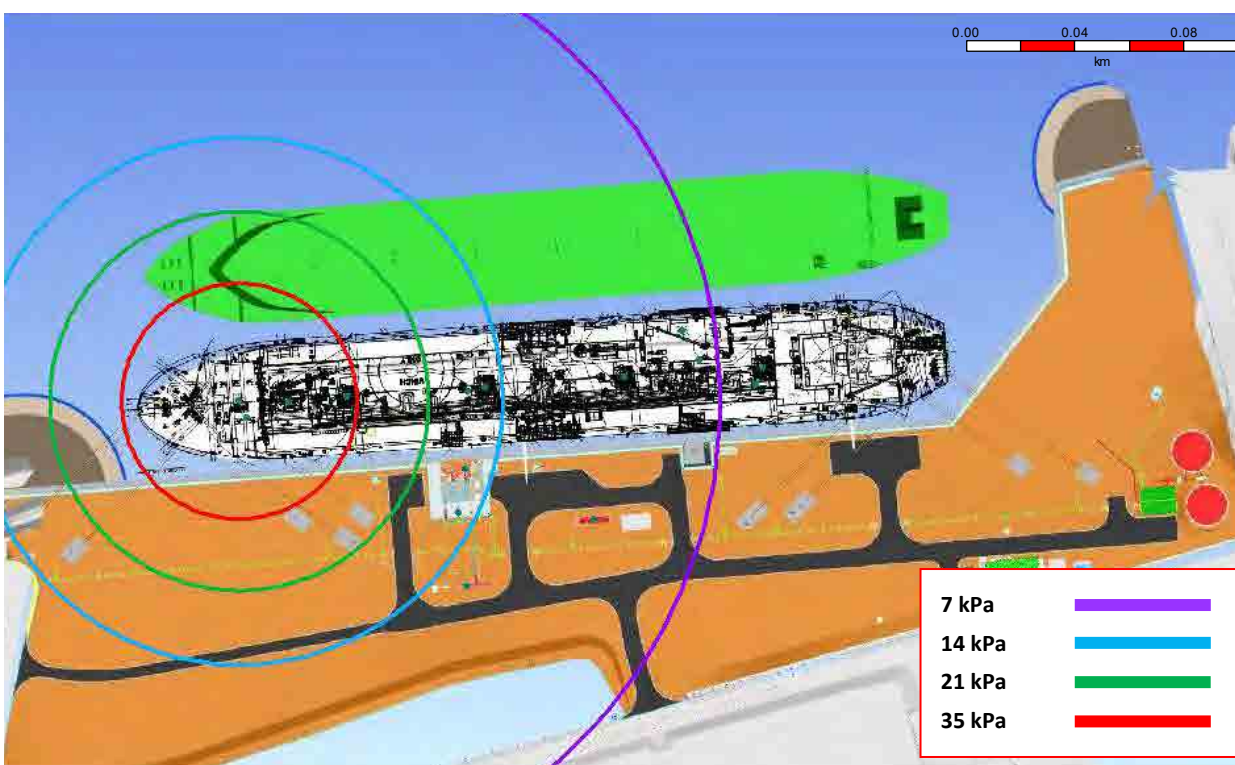
Figure 7-16: Regasification module (top half) VCE
