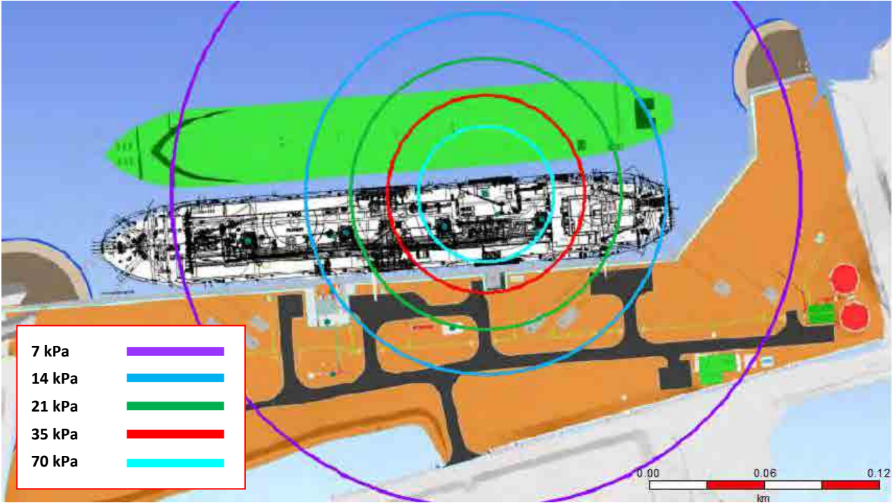
Figure 7-14: Cargo machinery room VCE
