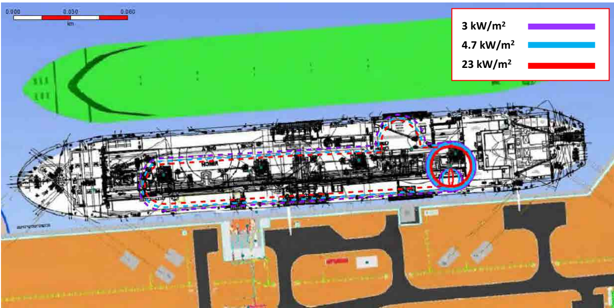
Figure 7-5: Scenario 3, 25mm Jet Fire Thermal Radiation Impacts at FSRU (14m above grade) – Initial Conditions
