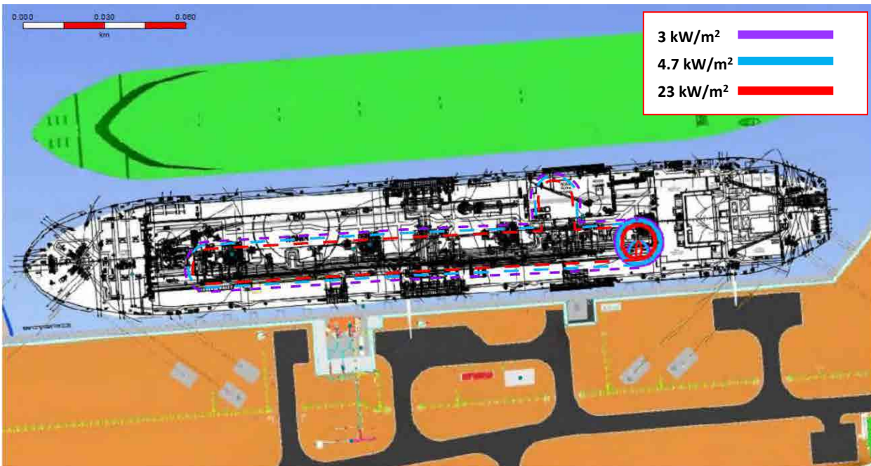
Figure 7-1: Scenario 1, 25mm Jet Fire Thermal Radiation Impacts at FSRU (14m above grade) – Initial Conditions
