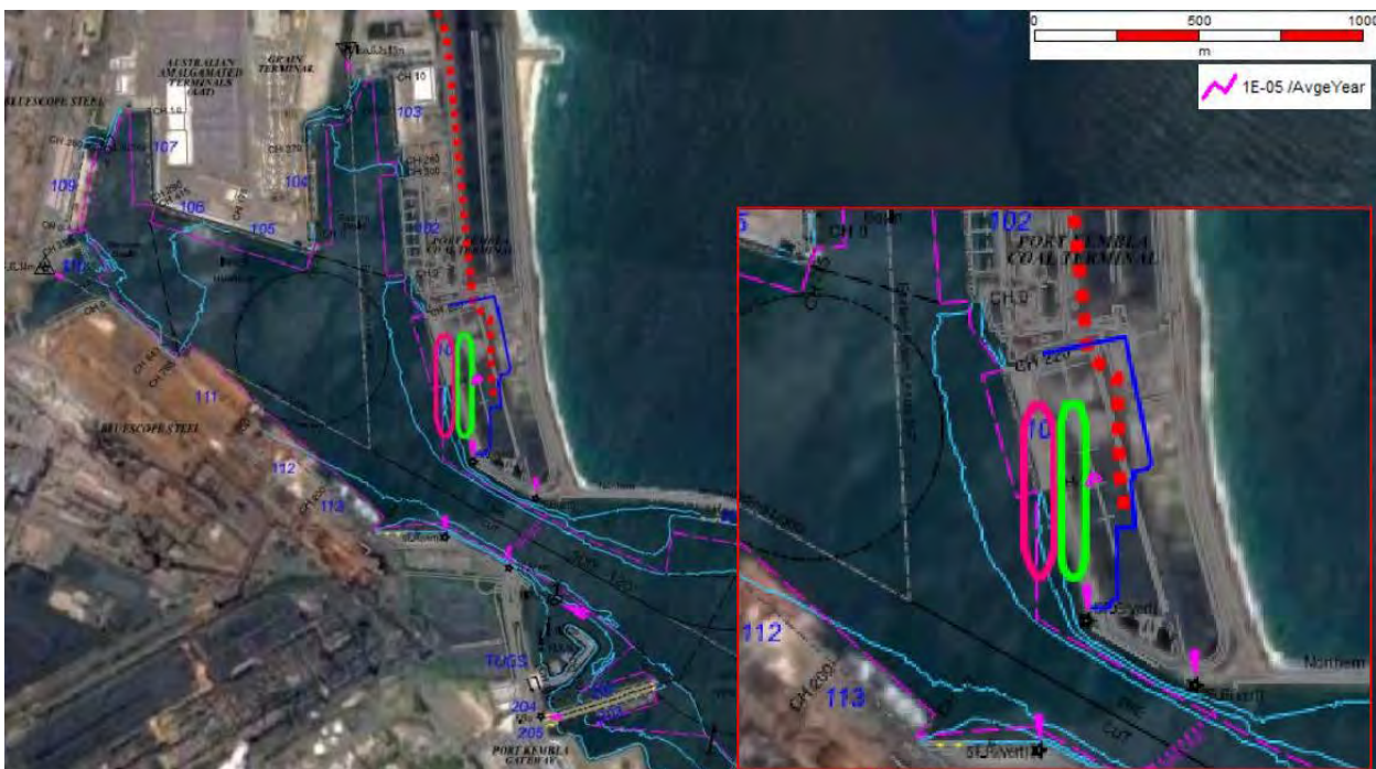
Figure 8-12: Injury Risk (1E-05 pa) - Serious injury due to toxic exposure (AEG2, 30 min)
