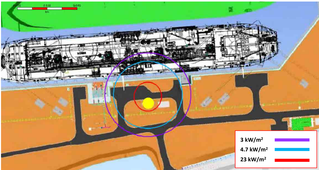
Figure 8-8: Scenario 9a, 25mm Pool Fire Thermal Radiation Impacts at ORF (1m above grade) – Initial Conditions
