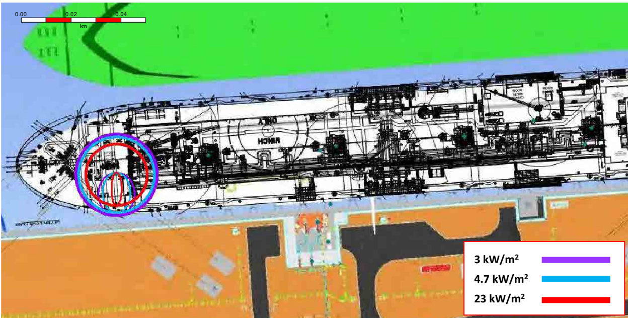
Figure 7-7: Scenario 4, 25mm Jet Fire Thermal Radiation Impacts at FSRU (14m above grade) – 5 minutes post release
