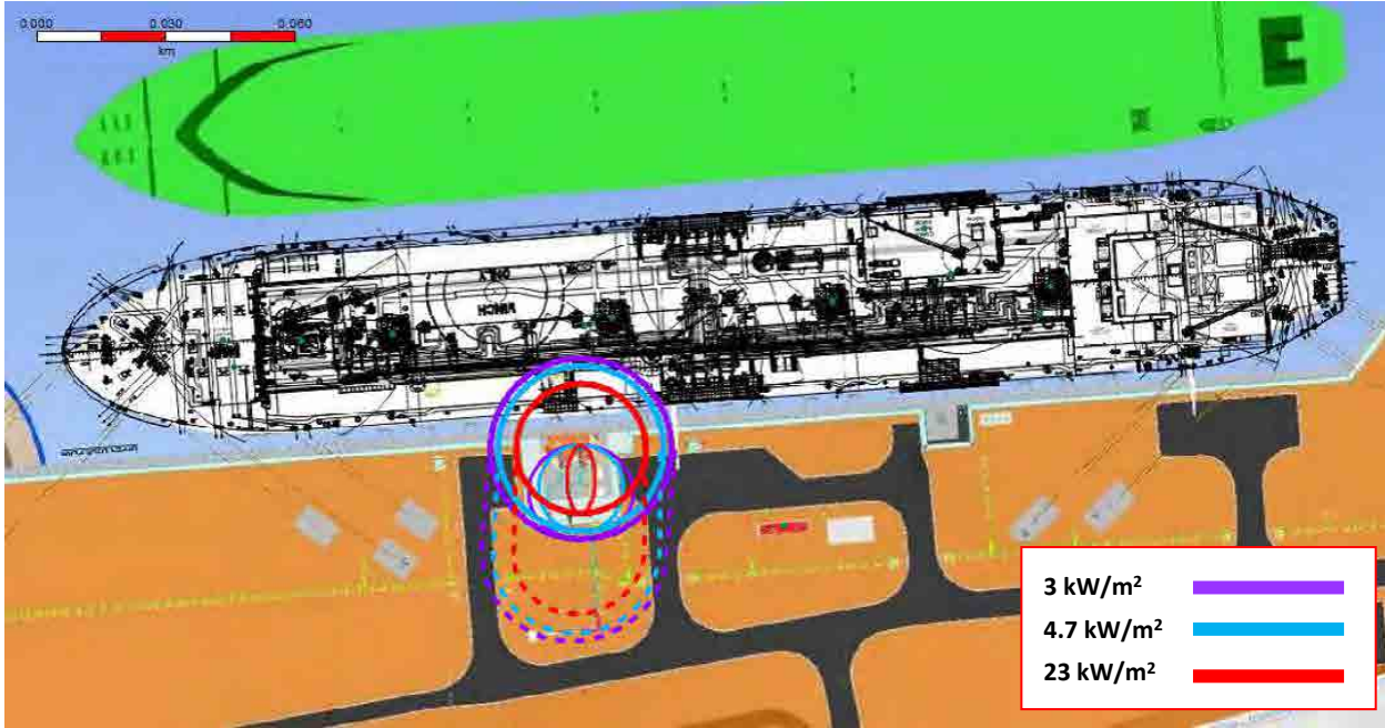
Figure 8-2: Scenario 6, 25mm Jet Fire Thermal Radiation Impacts at ORF (1m above grade) – After 5 Minutes
