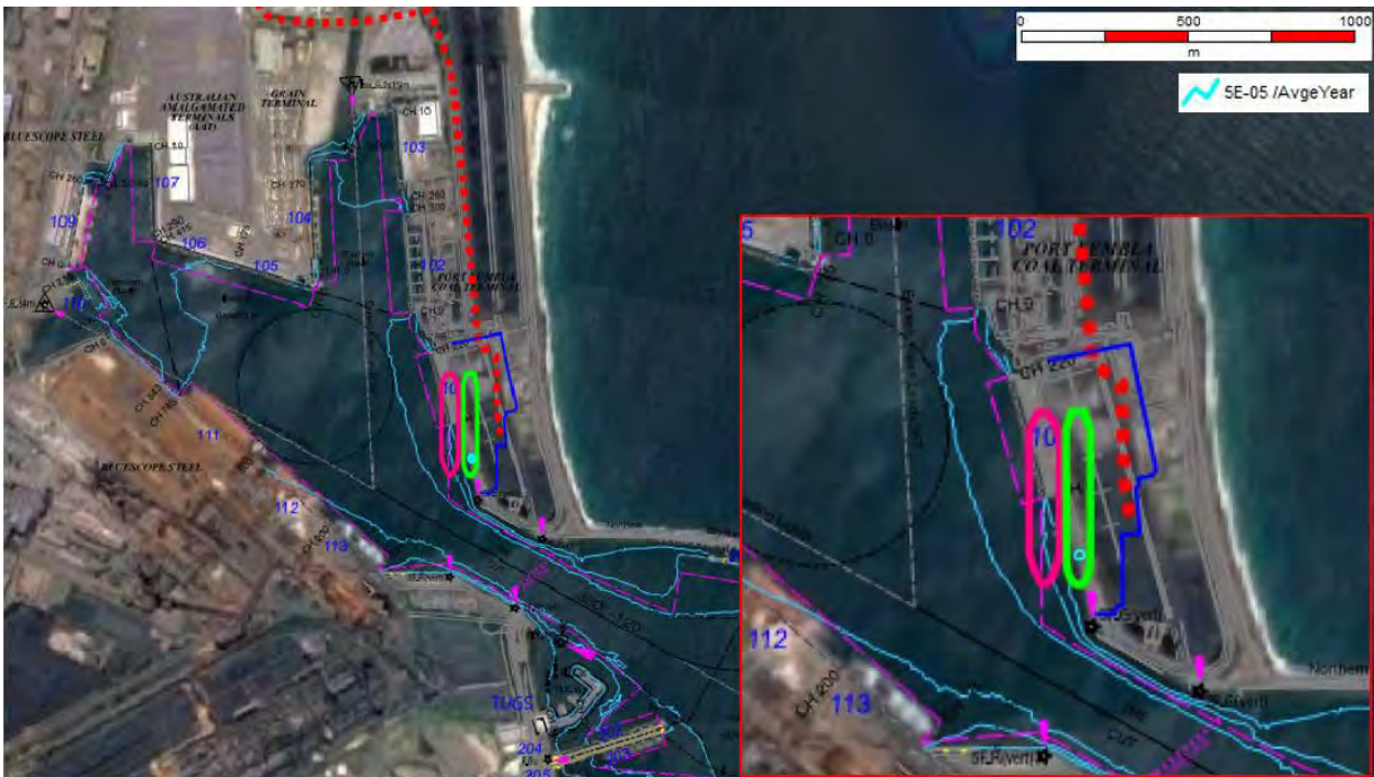
Figure 7-17: Property Damage (5E-05 pa) from 14 kPa Explosion Overpressure Levels
