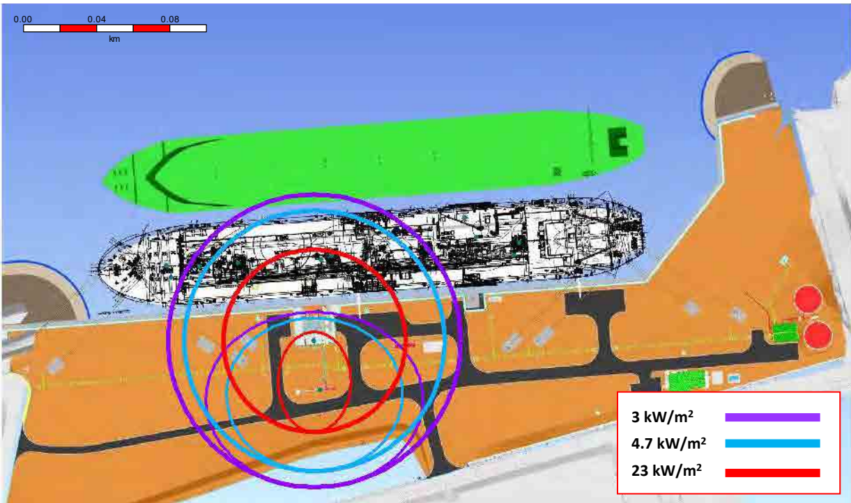
Figure 8-3: Scenario 7, 25mm Jet Fire Thermal Radiation Impacts at ORF (1m above grade) – Initial Conditions
