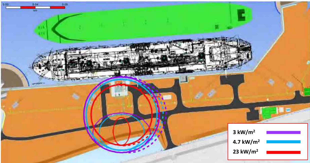
Figure 8-6: Scenario 8, 25mm Jet Fire Thermal Radiation Impacts at ORF (1m above grade) – After 5 Minutes
