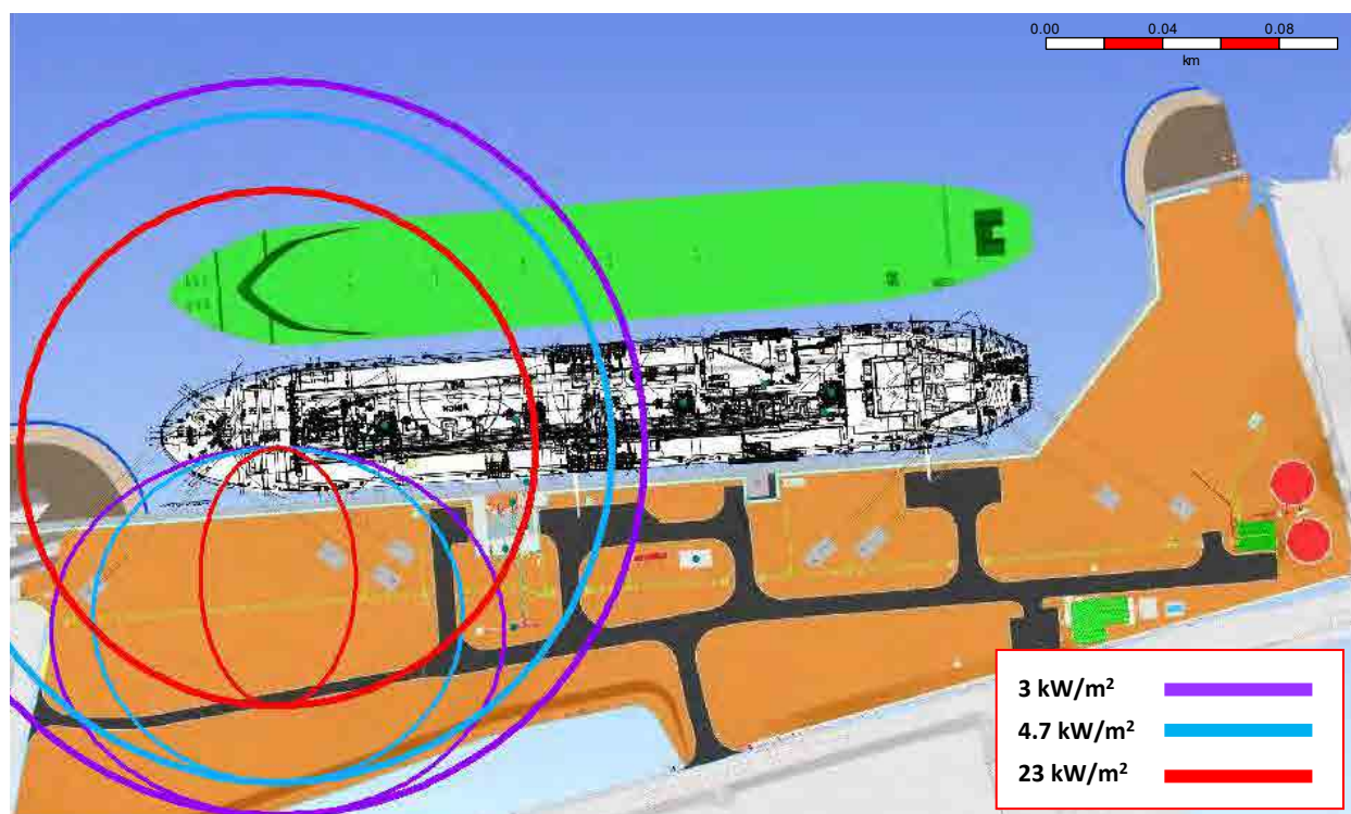
Figure 7-6: Scenario 4, 25mm Jet Fire Thermal Radiation Impacts at FSRU (14m above grade) – Initial Conditions
