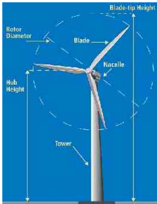
Configuration and components of a typical wind turbine
