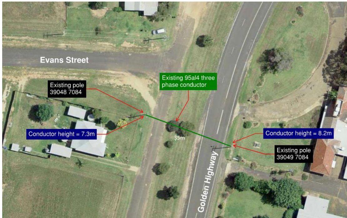
Figure 19 – Golden Highway & Evans Street conductor arrangement
