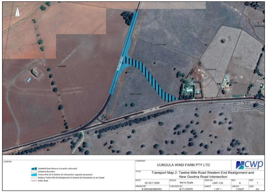
Figure 3 | Twelve Mile Road / Goolma Road Realignment and Intersection
